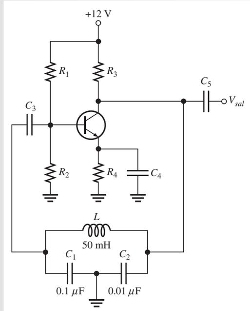
**Solución** (a)  $C_T = \frac{C_1 C_2}{C_1 + C_2} = \frac{(0.1 \mu\text{F})(0.01 \mu\text{F})}{0.11 \mu\text{F}} = 0.0091 \mu\text{F}$
