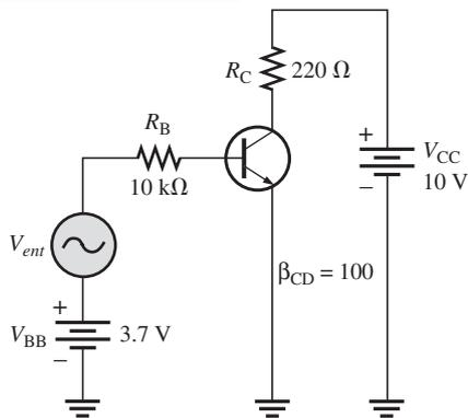
$$I_{BQ} = \frac{V_{BB} - 0.7 \text{ V}}{R_B} = \frac{3.7 \text{ V} - 0.7 \text{ V}}{10 \text{ k}\Omega} = 300 \mu\text{A}$$
