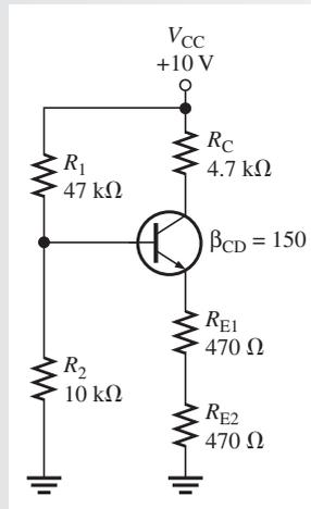
$$R_{\text{ENT(BASE)}} = \beta_{\text{CD}}(R_{\text{E1}} + R_{\text{E2}}) = 150(940 \Omega) = 141 \text{ k}\Omega$$
