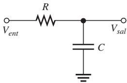
$$\frac{V_{sal}}{V_{ent}} = \frac{X_C}{\sqrt{R^2 + X_C^2}}$$
