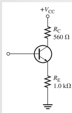
**Solución**  $R_{ENT(BASE)} = \beta_{CD}R_E = (125)(1.0 \text{ k}\Omega) = 125 \text{ k}\Omega$
