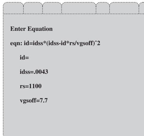
The image shows a TI-86 calculator screen with a grey background and a dotted border. At the top, there are several small, rounded rectangular buttons. Below them, the text "Enter Equation" is displayed. The equation  $eqn: id=idss*(idss-id*rs/vgsoff)^2$  is shown. Below the equation, the variables are listed:  $id=$ ,  $idss=.0043$ ,  $rs=1100$ , and  $vgsoff=7.7$ .
